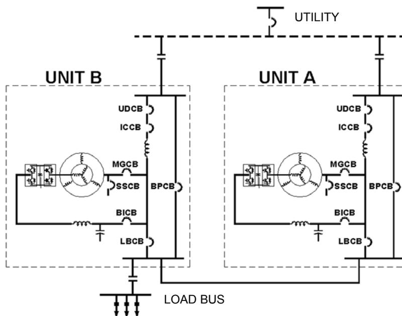
Figure 1-2. Parallel N+1 Redundant Unit System [N=1]
