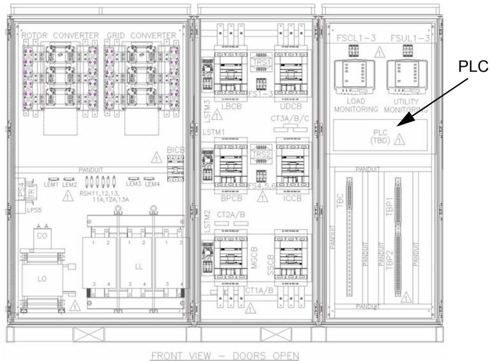
**Figure 4-3. Location of the PLC for the 315 kVA System**
