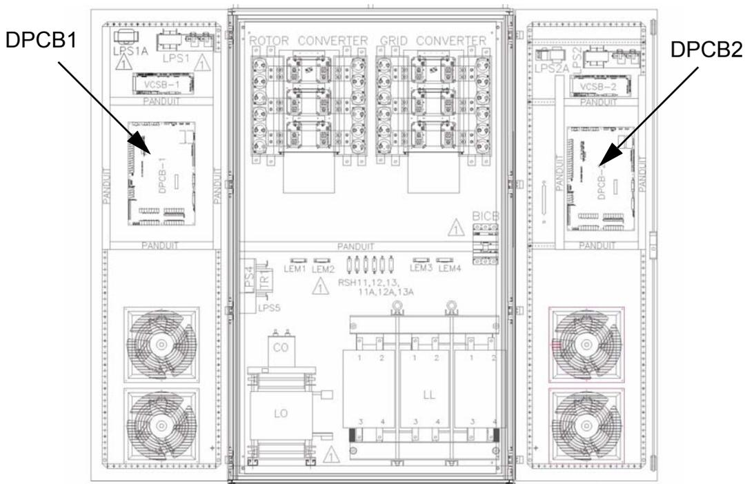
Figure 4-2. Location of DPCB1 and DPCB2 for the 315 kVA System
