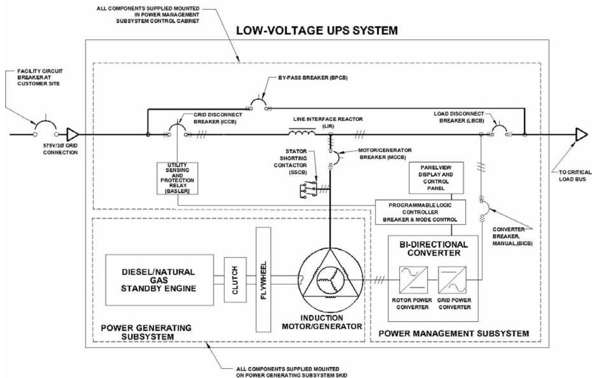
Figure 1-1. UPS System One-line Diagram
