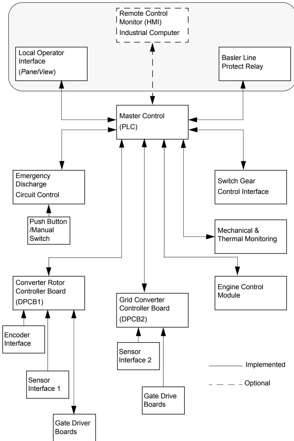
**Figure 1-3. UPS Control Block Diagram**
